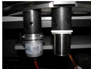
(b) Baffle motor and encoder
