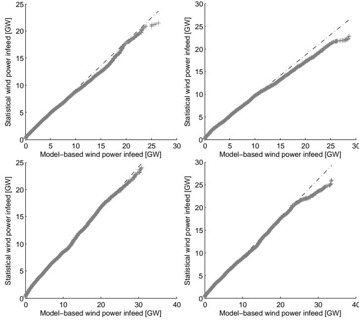
Figure 3.8: QQ-plots of model-based and historical production profiles, for the years 2010-2013
