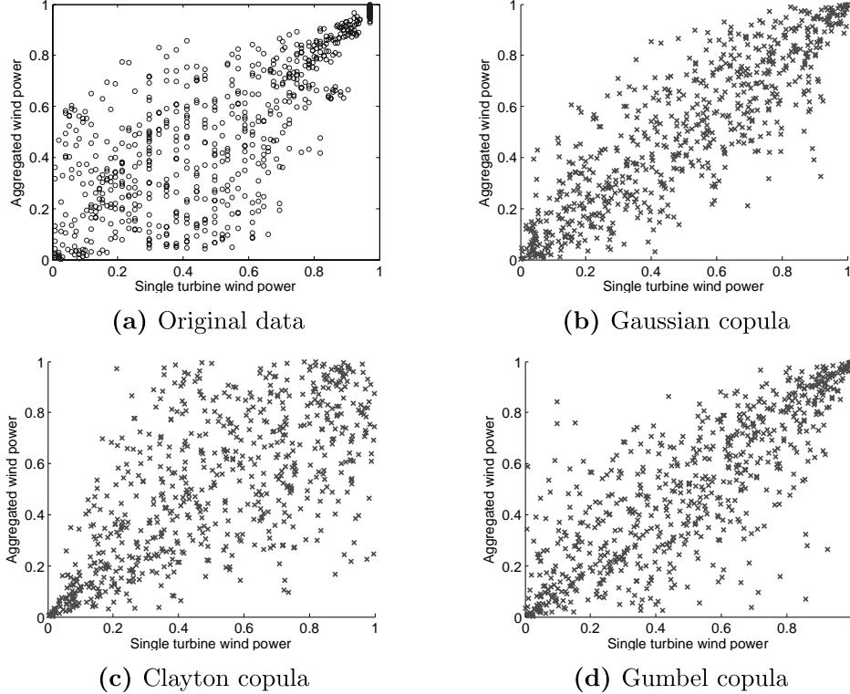
Figure 2.3: Dependence structure of the original data and simulations from three copula models
