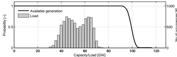
Figure 3.1: Complementary cdf of Germany's power plants without wind power together with a histogram of 2013 load levels
