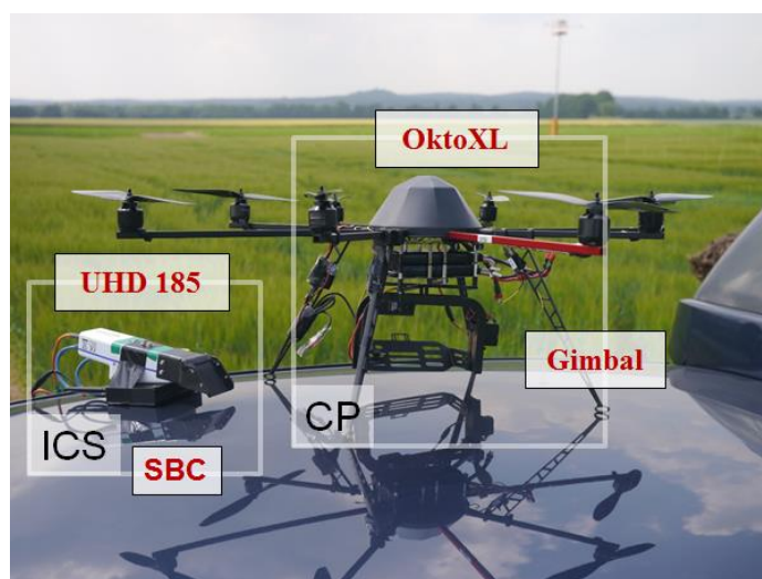
Figure 3.1 Carrier Platform (CP) MikroCopter Okto XL with Gimbal and image capturing system (ICS) with UHD 185-Firefly and the single board computer (SBC) Pokini Z.
