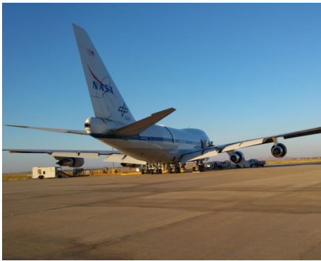
Figure 2.4.1.: The Boeing 747sp aircraft turned into the airborne observatory SOFIA. Photo: M. Mertens
