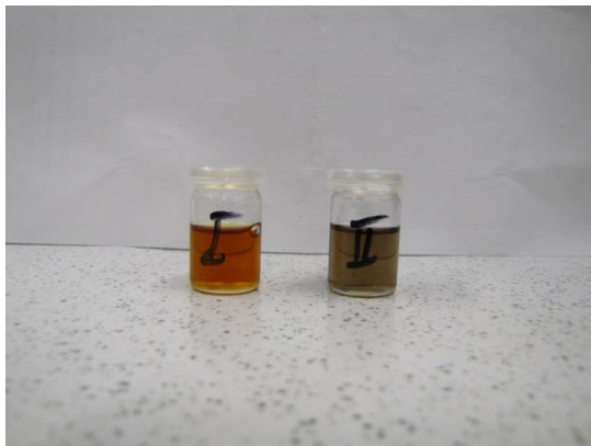
Figure 5-19. Visible color change for the destabilized sample (II), caused by Ag agglomeration.
