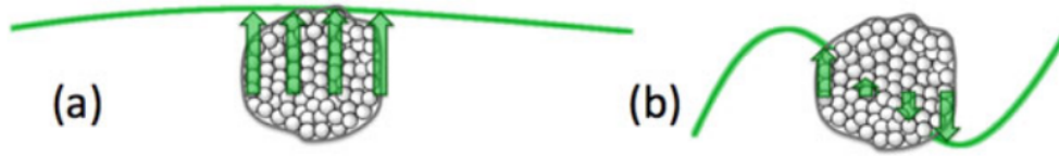
Figure 2.7: Schematic drawing showing a particle smaller than the wavelength (a) and a particle large compared to the wavelength (b). The white spheres in the particles illustrate the dipoles, the green line the EM wave and the arrows the induced field. In (a) all dipoles oscillate in phase with each other, while in panel (b), the dipoles oscillate out of phase, thus reducing the backscattered signal. This graphic is taken from Kumjian, 2018 with permission from Springer Nature under license number 5372471325791
