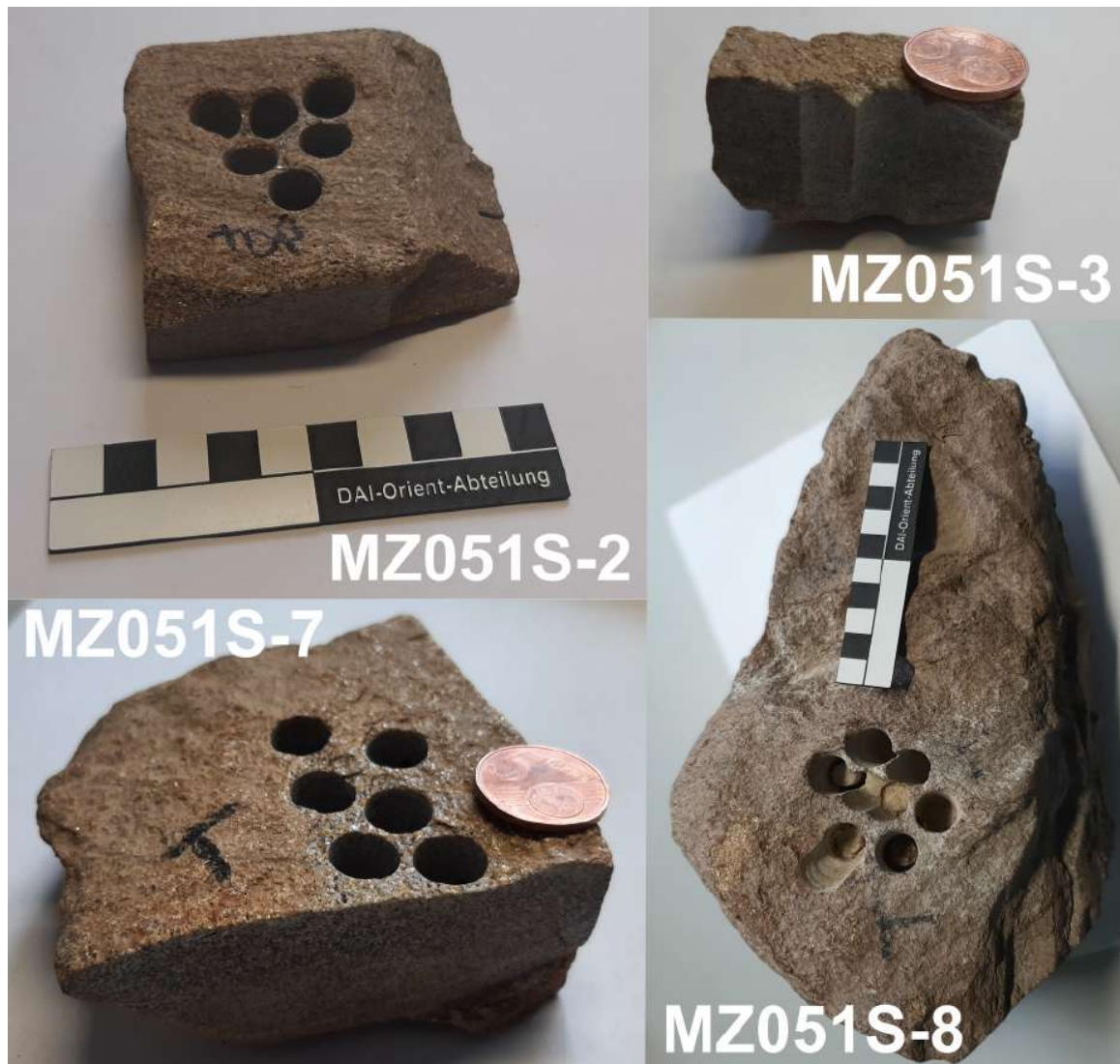
Fig. B.2: The dated cobbles from MZ051S. MZ051S-2, MZ051S-7 and MZ051S-8 are paragneisses; MZ051S-3 is an orthogneiss. The pictures are taken after material (approximately 200 grams) has been removed for dose rate measurements (gamma spectrometry).
