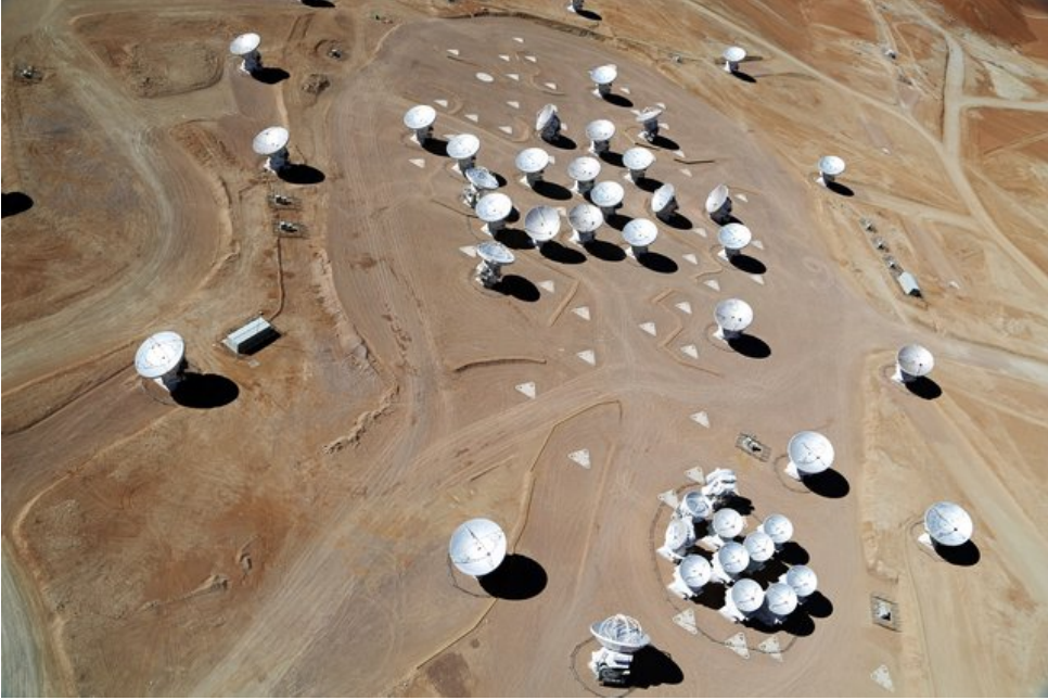
Figure 3.1.: The compact array and a part of the 12-meter array in the aerial image of the ALMA interferometer Credit: Clem & Adri Bacri-Normier
