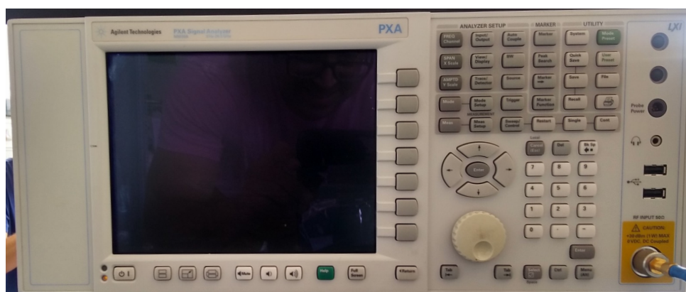
Figure 4.17: Agilent Technologies PXA Spectrum analyzer N9030A used to record the IF band of the IBAMI. The input is connected to an Agilent power meter that receives the combined outputs of the IBAMI.
