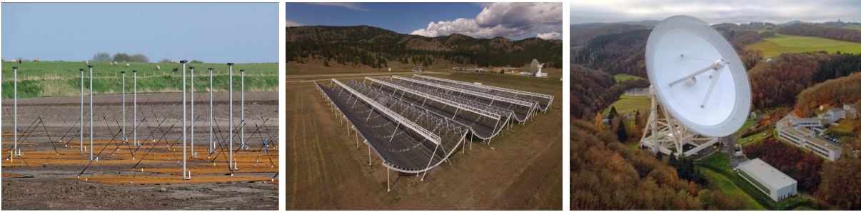
Figure 4.1: The three types of antennas used for astronomical observations: a , LOFAR dipole antennas; b , wire mesh antennas of CHIME; c , the Effelsberg 100-m parabola antenna. Image credits: ASTRON, CHIME, MPIfR/Norbert Tacken.
