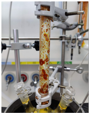
Figure 81: Picture of the sublimation tube during the reaction of NH_4Cl and S_2Cl_2 at 140\text{ }^\circ C . At this moment, the orange-brown solid already indicated the presence of (S_3N_2Cl)Cl .
