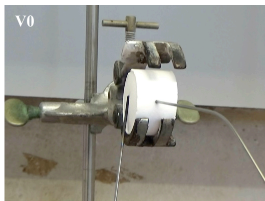
Figure 34: Photographic image of sample V0 before fire testing.
