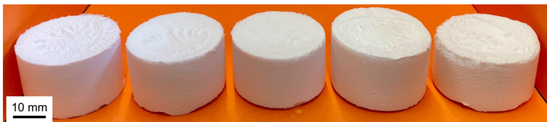
Figure A 1: Samples with increasing dilution of the precursor system (left to right). The sample dimensions are around 35 mm in diameter.
