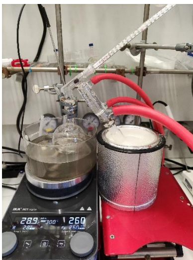
Figure 50. Distillation of the non-reacted styrene under vacuum.
