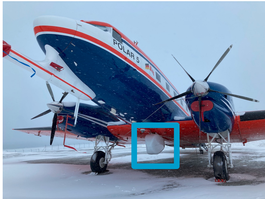
Figure 1.3: Microwave Radar/radiometer for Arctic Clouds (MiRAC) mounted within the belly pod under the research aircraft Polar 5 . The picture was taken by Pavel Krobot.
