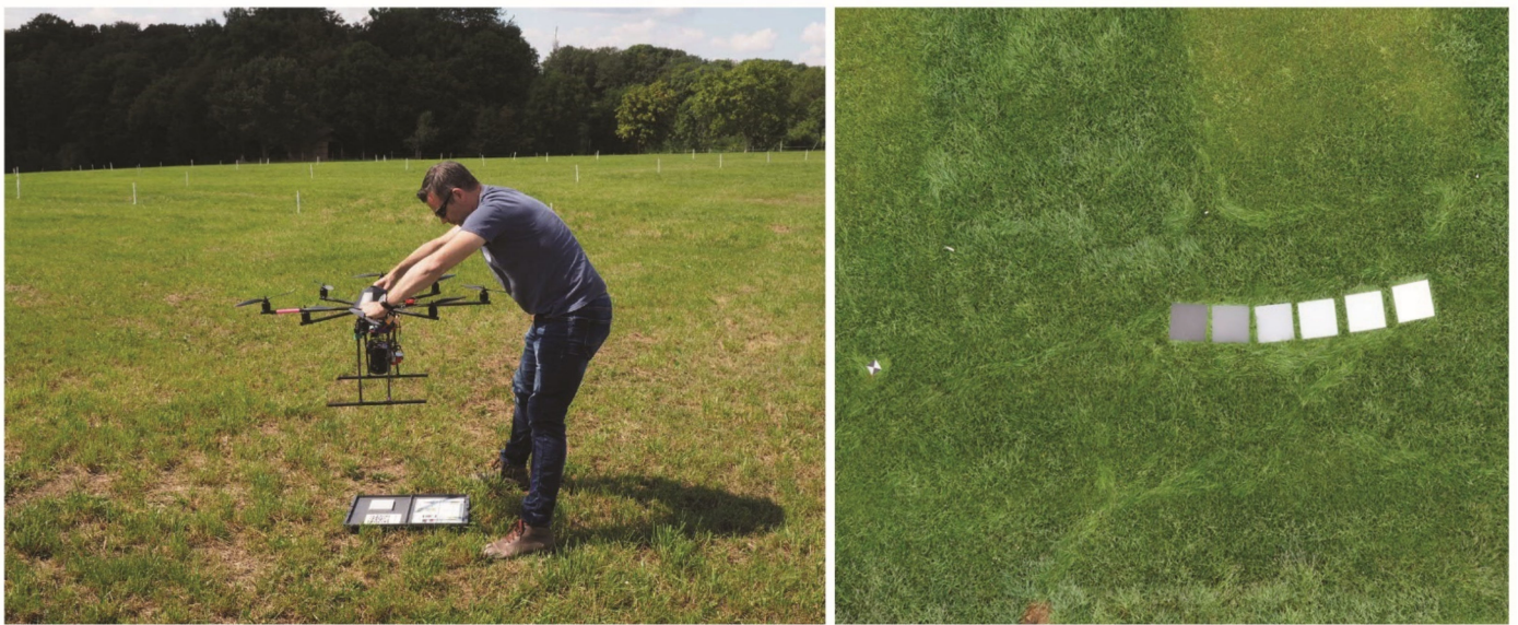
Figure 5. Acquiring images of the MicaSense RedEdge-M radiometric calibration panel ((left); image credits: Christoph Hütt), and additional gray panels for radiometric assessment and ground control point (right).
