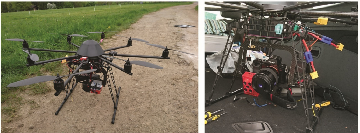
Figure 4. Multirotor UAV equipped with MicaSense RedEdge-M and Sony Alpha 7r cameras.
