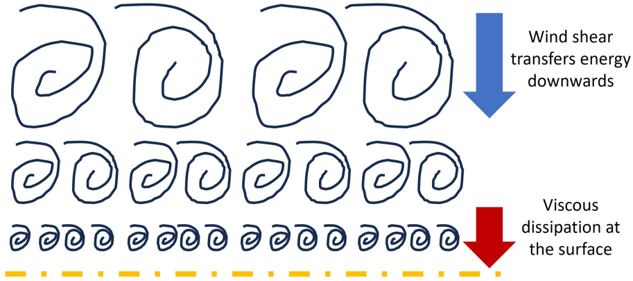
Figure 2.7: The general energy dissipation scheme in turbulent flow where larger eddies transfer energy into smaller ones in cascading manner until it is dissipated at the bed surface.
