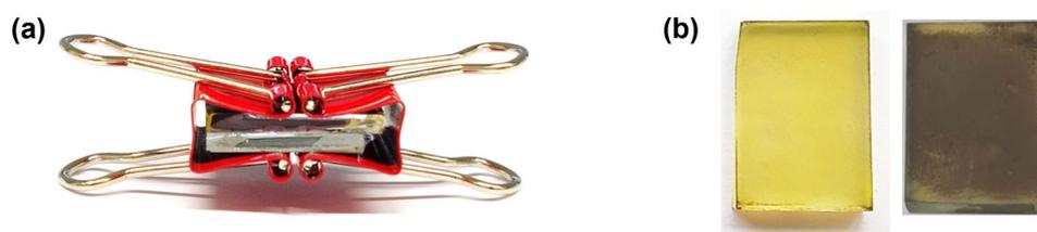
**Figure 1.** (a) Perovskite-coated substrate in physical contact for PCA. (b) color change of the FAPbI<sub>3</sub> sample from yellow (as-prepared) to grey (after 20 h PCA).
