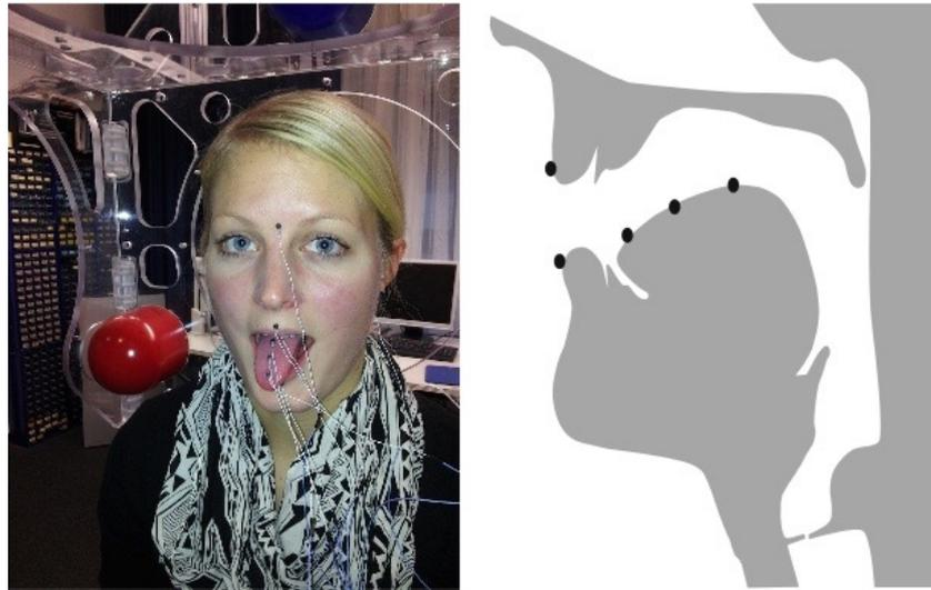
Figure 4.1: Position of the sensor coils attached to the subject's articulators.
