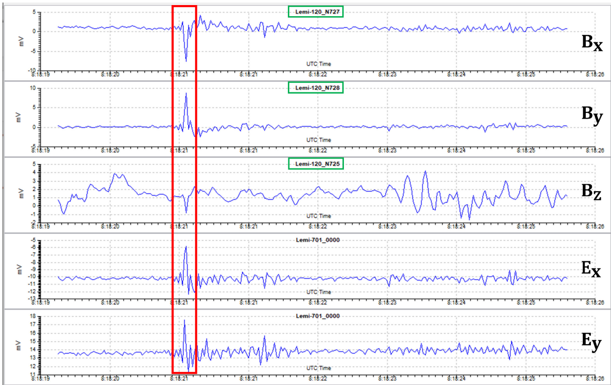
Figure 6.1: Example of unfiltered time series recorded at MT09 highlighting the correlation between B_y and E_x components and the anti-correlation between B_x and E_y . The sensor model and the serial number of each induction coil, which is related to the calibration factors, are also visible.
