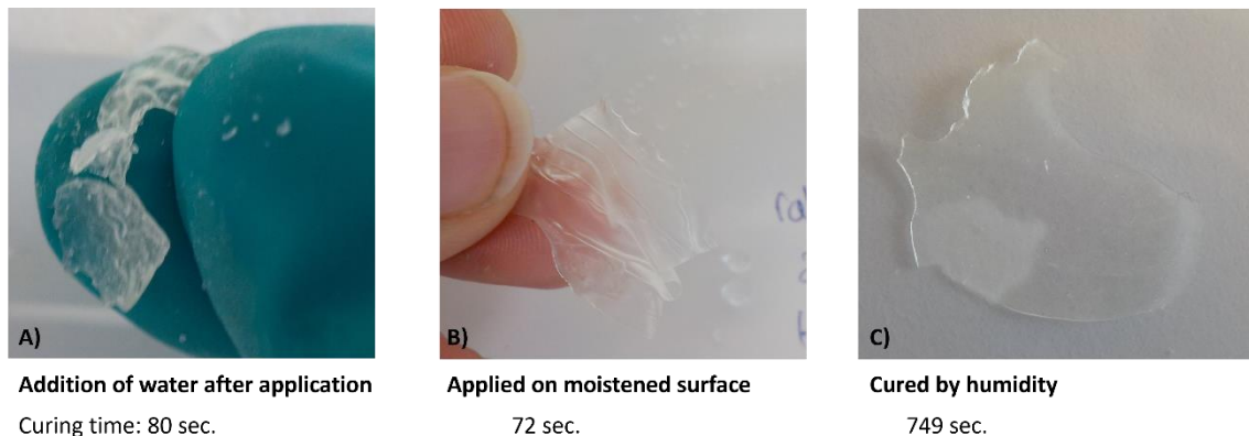
Figure 52 Cured materials from EtOSi-prepolymer-1 obtained by different curing approaches. A) Addition of water after the application B) applying EtOSi-prepolymer-1 on a moistened surface C) cured by humidity. Curing times are given for each approach defined here as the time taken until no more material sticks to the gloves when touching the film.
