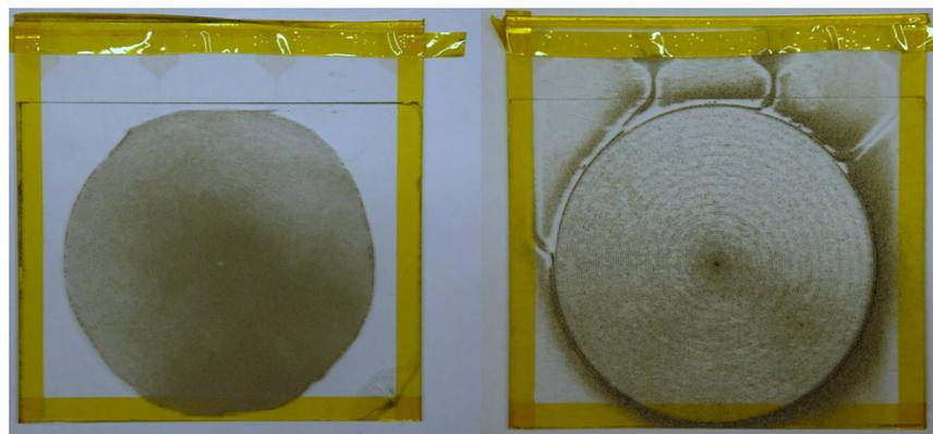
Figure 7.11: Photographs showing EDS tests conducted under the same vacuum condition (no UV) with samples of LMS-1 25–50  $\mu\text{m}$  grains. Left: Unbaked sample, showing almost no particle displacement. Right: Baked sample.
