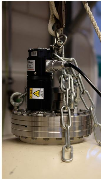
Figure 6.10: VUV lamp utilised for generating the photoelectric effect, positioned directly above one of the EDS plates. The lamp takes 25 sec to warm up and immediately outputs the maximum UV intensity.
