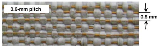
Figure 4.3: Insulated wire electrodes embedded in a spacesuit material, from Kawamoto et al. (2011a).
