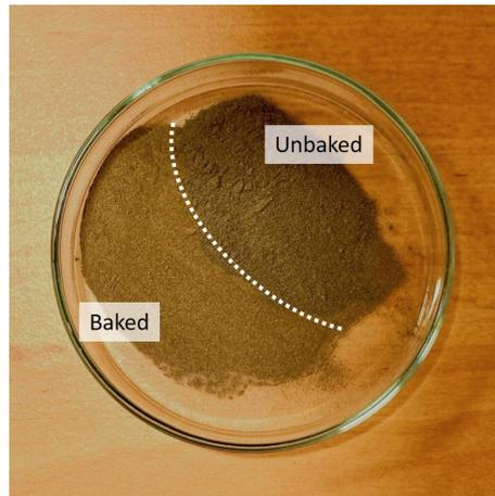
Figure 6.5: Simulant samples (LMS-1 in 25–50  $\mu\text{m}$  size range) in a Petri dish that usually goes into the vacuum oven for baking. Here some unbaked grains are placed next to the baked grains for comparison. A visible colour difference due to moisture content can be observed.
