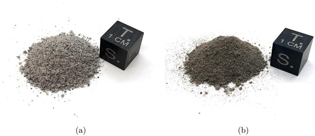
Figure 3.4: (a) Sample of LHS-1. (b) Sample of LMS-1. Source: University of Central Florida.
