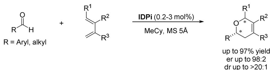
**Scheme 4.29** Asymmetric catalytic HDA reaction.
