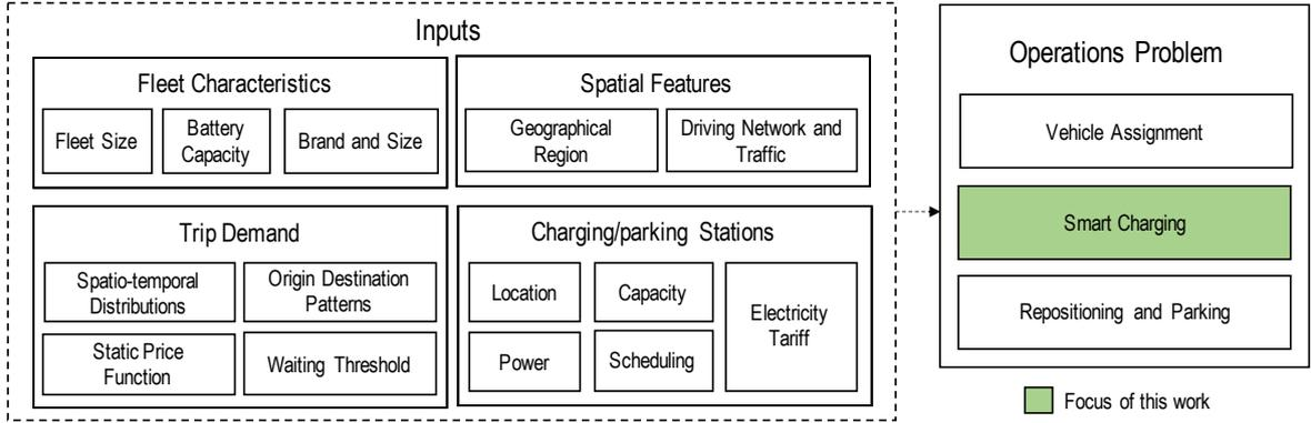
**Figure 2.1:** Operations Problem of a Shared Autonomous Electric Fleet
