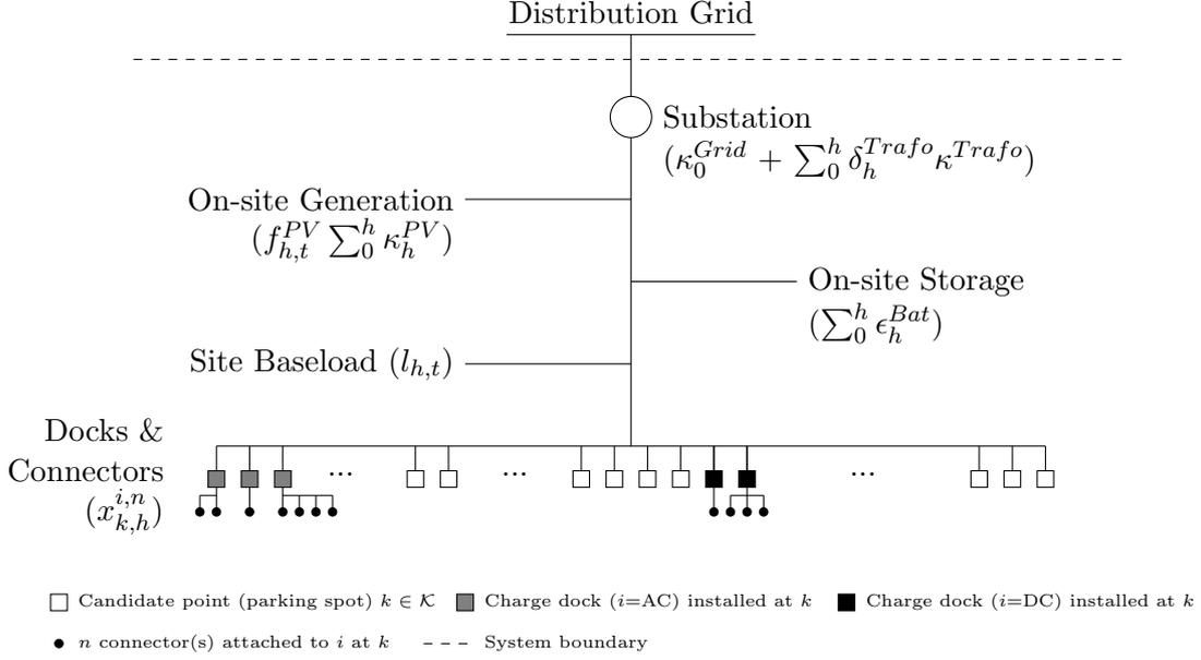
**Figure 4.2:** EVCH Service System Layout and Asset Components in Planning Stage  $h$
