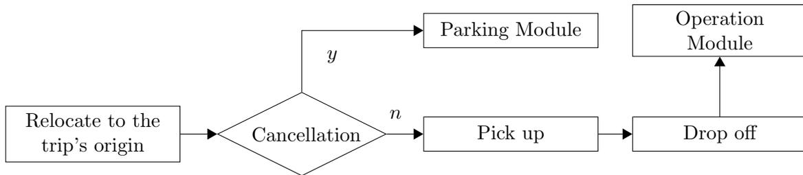
**Figure 2.14:** Trip Module of SAEVs: the Process of Serving a Trip after Matching to a Vehicle
