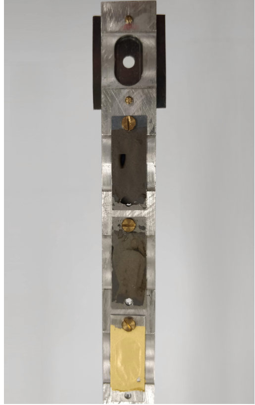
(b) The target ladder with (top to bottom) a 3 mm diameter aperture, the two ^{nat}\text{C} , and the ^{197}\text{Au} target. The used target shows the darkened beam spot.
