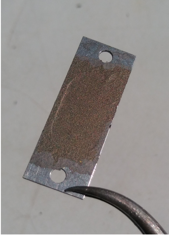
(a) The 0.114 \frac{\text{mg}}{\text{cm}^2} ^{nat}\text{C} target which was used in both beam times, glued onto an aluminum support frame before being mounted onto the target ladder assembly.
