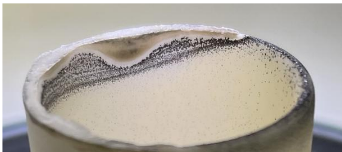
Figure 5.10: Formation of black crystallites on the upper inner crucible wall (experiment S-ID 3), indicating gas-phase transport during the synthesis process.
