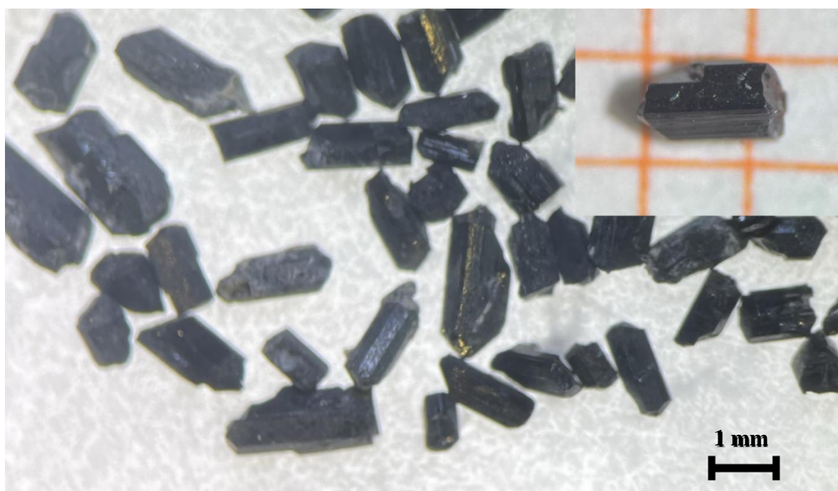
Figure 6.1: \text{Ba}_4\text{Ir}_3\text{O}_{10} single crystals obtained from \text{BaCl}_2 flux growth, exhibiting well-defined morphology and sizes in the millimeter range. Scale bar: 1 mm
