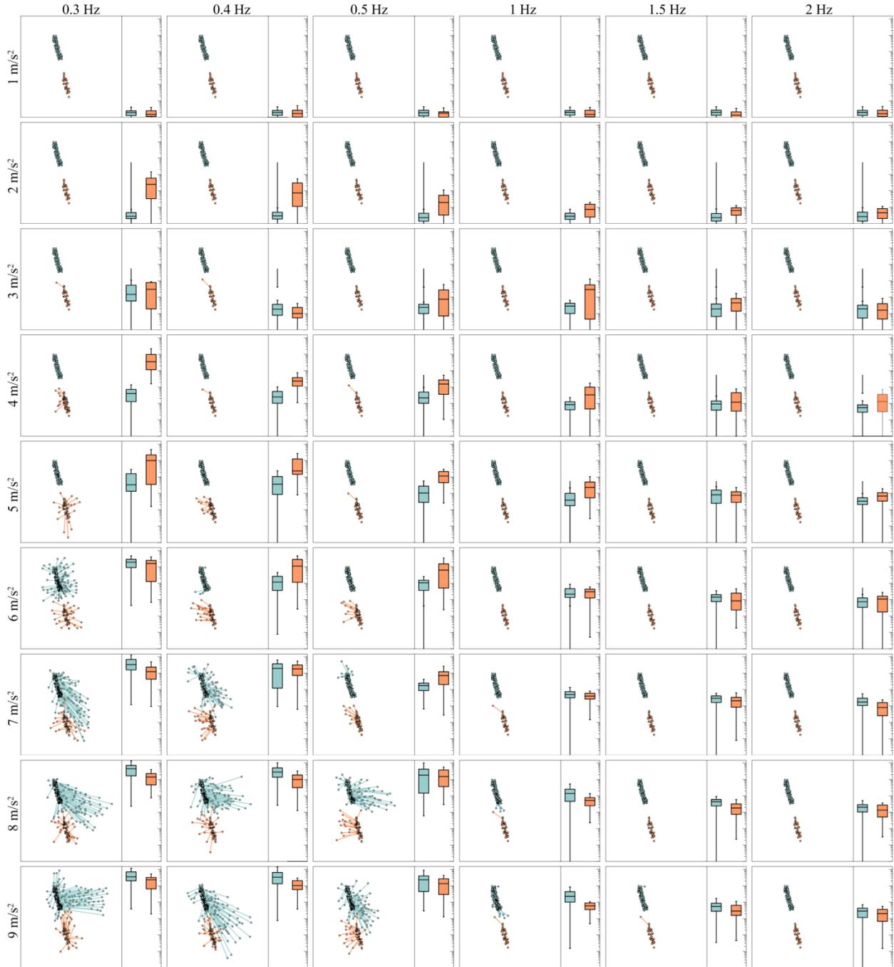
Figure 5.11: The results of horizontal ground motions parallel (top to bottom) to the wall trend. Rows and columns give the PGA and main frequency of the pulses, respectively, as indicated at the left and top border. Each individual graph has the same scaling as the graphs in Figure 5.9 (Schweppe et al. 2017).
