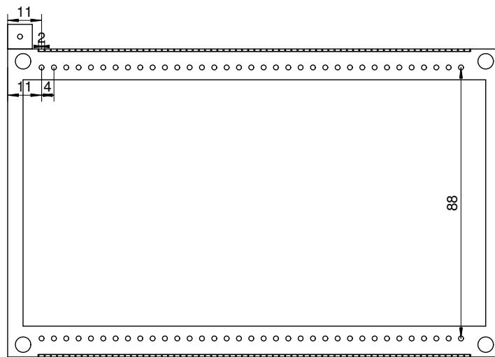
(a) Top view of the first design of the anode board. First two anodes are split diagonally.
